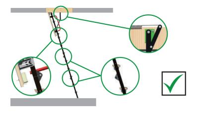
Check that the ladder unfolds properly. When unfolded, individual segments of the ladder must adjoin each other and form a straight line, and the upper arms must lie against the limiters.
