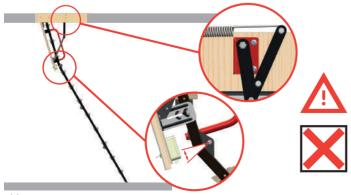
If the stairs are too long, the ladder segments do not form a straight line, and the upper arms do not lie against the limiters, then you must cut the ladder according to the next steps.
