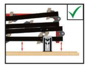
Make sure the ladder is screwed securely. The ladder must be mounted in the highest possible position.
