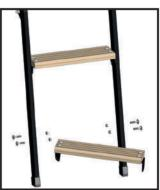
**Step 28**If the cut line is at this point, remove the step.
