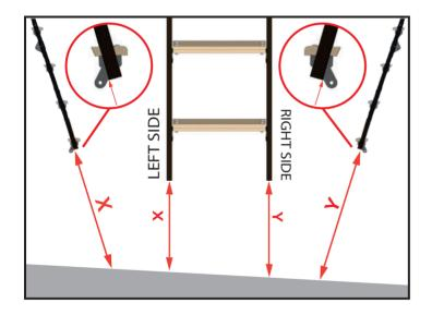
**Step 26** Measure the X dimension from the outer end (at the left hinge) of the wooden section to the floor. Then subtract 0.2 in (foot size) from the X dimension. Measure and mark this dimension on the last segment. Repeat for the Y dimension (right side of the ladder).
