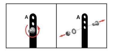
Step 9 Remove the nuts and remove the washers and screws from arms A.
