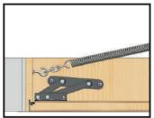
**Step 8**Stretch the springs and attach them to the chains according to the table below.
