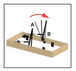
Place arm B in a vertical position, then stretch arm A so that it gets closer to arm B. Then screw arms A and B together at the marked positions. Remember to put the washer between the arms. Screw the arms tightly, but only use 90% of the force. The arms should be screwed in the mounting holes in accordance with the model of stairs installed by you.
